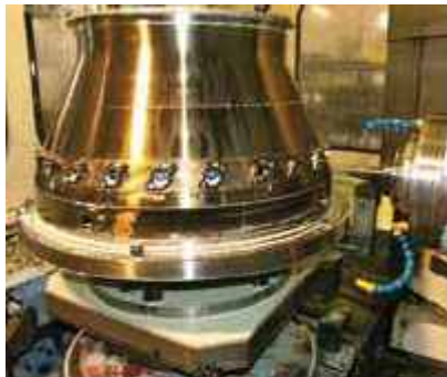
Seco's Threadmaster saved two-thirds of the thread milling time on a combustor case component made of Inconel 718 heat-treated to R C 42 at Gentz Industries.
