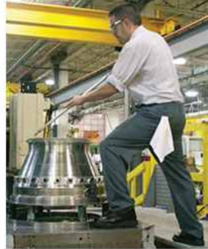
Using its Productivity Cost Analysis program, Seco is now studying the other operations performed on the combustor case including turning, rough milling, debossing, heat treating, and finish milling.
